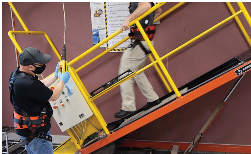
The “German Ramp” test, standardized in DIN EN 16165. Credit: TCNA.
