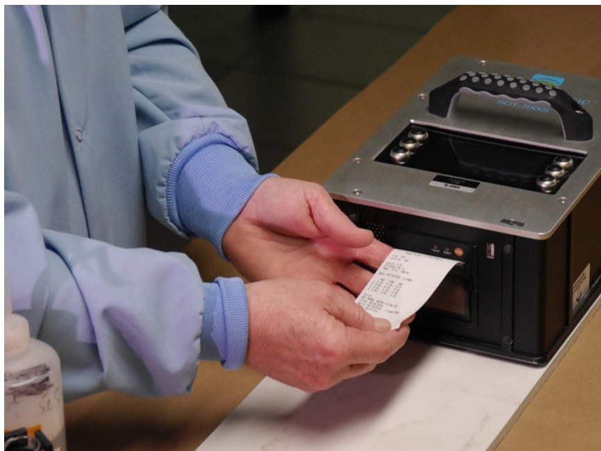
A BOT 3000E device, commonly used to measure DCOF. Credit: TCNA.
